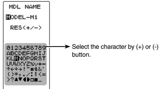
Also move the cursor to "RES<+/->" by (UP) or (DN) button and press the (+) and (-) buttons simultaneously for approximately 1 second. A beeping sound is generated and the model name is initialized to the factory setting.
