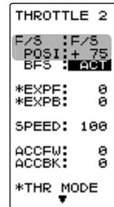
When the receiver power supply of an electric car uses a common power supply from an ESC, we recommend that this function be set to OFF because the voltage supplied to the receiver may drop momentarily and the battery fail safe function may be activated.
