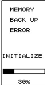
If the data is lost for an unknown reason, an audible alarm will sound and "MEMORY BACK UP ERROR" will be displayed on the LCD screen.
