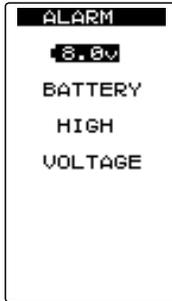
If a battery exceeding 8V is used with the T4PL, an audible alarm will sound and "BATTERY HIGH VOLTAGE" will be displayed on the LCD screen.
