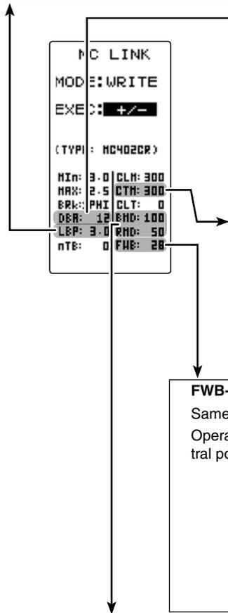
**CTM-(C.L. TIME LIMIT) 50A~300A /CLT-(C.L. TIMER) 0sec(OFF)~240sec (except MC950CR)**
