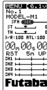
"HIGH" is displayed for high speed type and nothing is displayed for normal type.
