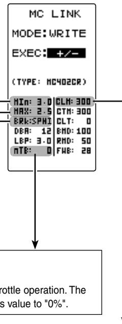
"Min" which sets the frequency when the load is small, is set to the high frequency side (large value) when extension is desired after straight-aways and curves.
