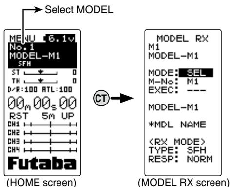
On the HOME screen, open the MENU screen by selecting MENU by (UP) or (DN) button and pressing the (CT) button. Next, display the MODEL RX screen by selecting MODEL RX by (UP) or (DN) button and pressing the (CT) button.
